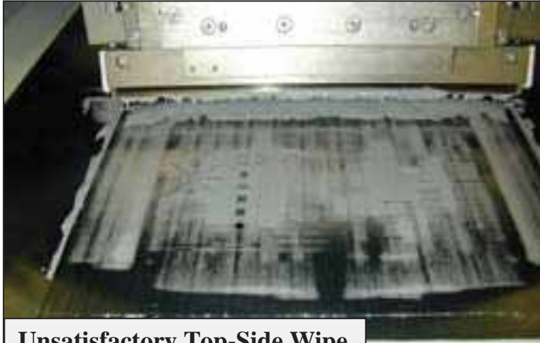
Unsatisfactory Top-Side Wipe
